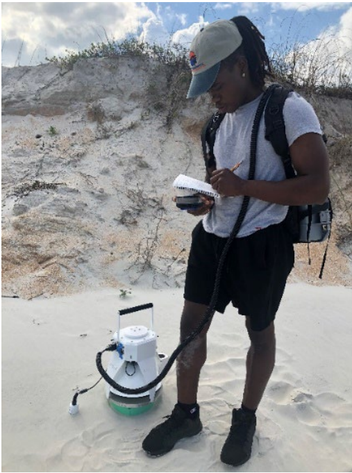
Jaren Serano measures gas efflux at the dune toe of a beach. RAYMOND CARTHY
