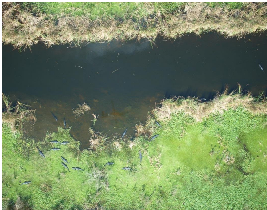
Image from low level flight of the South Florida Wildlife Management's Bell 407 equipped with the UAS payload mounted on the step. Features such as altitude, gps location, transect width, and alligator length, are measureable in the geo-referenced image.
