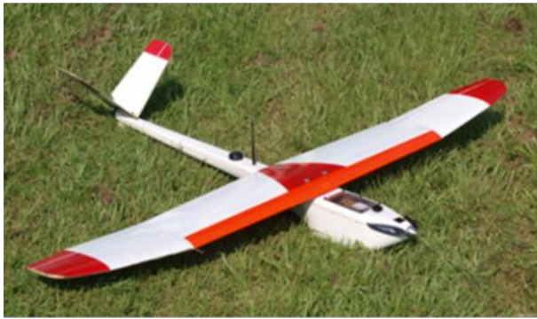
Figure 1. The NOVA 2.1 can be hand launched and landed on land or water.
