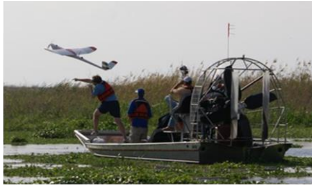
Figure 1. The NOVA 2.1 can be hand launched and landed on land or water.
