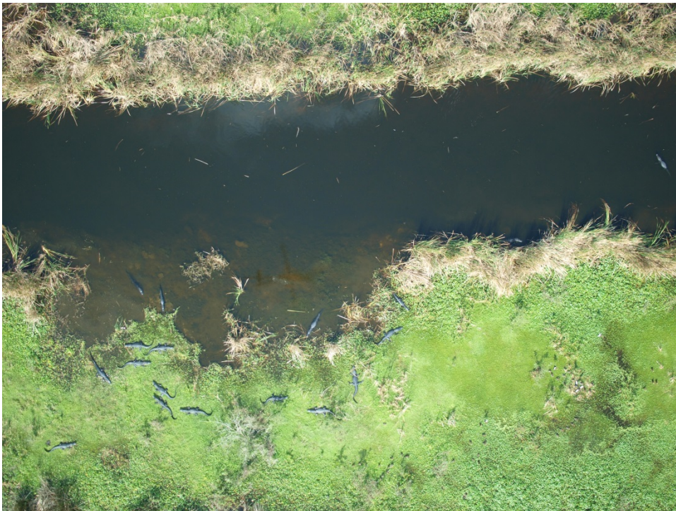
Image from low level flight of the South Florida Wildlife Management’s Bell 407 equipped with the UAS payload mounted on the step. Features such as altitude, gps location, transect width, and alligator length, are measureable in the geo-referenced image.
